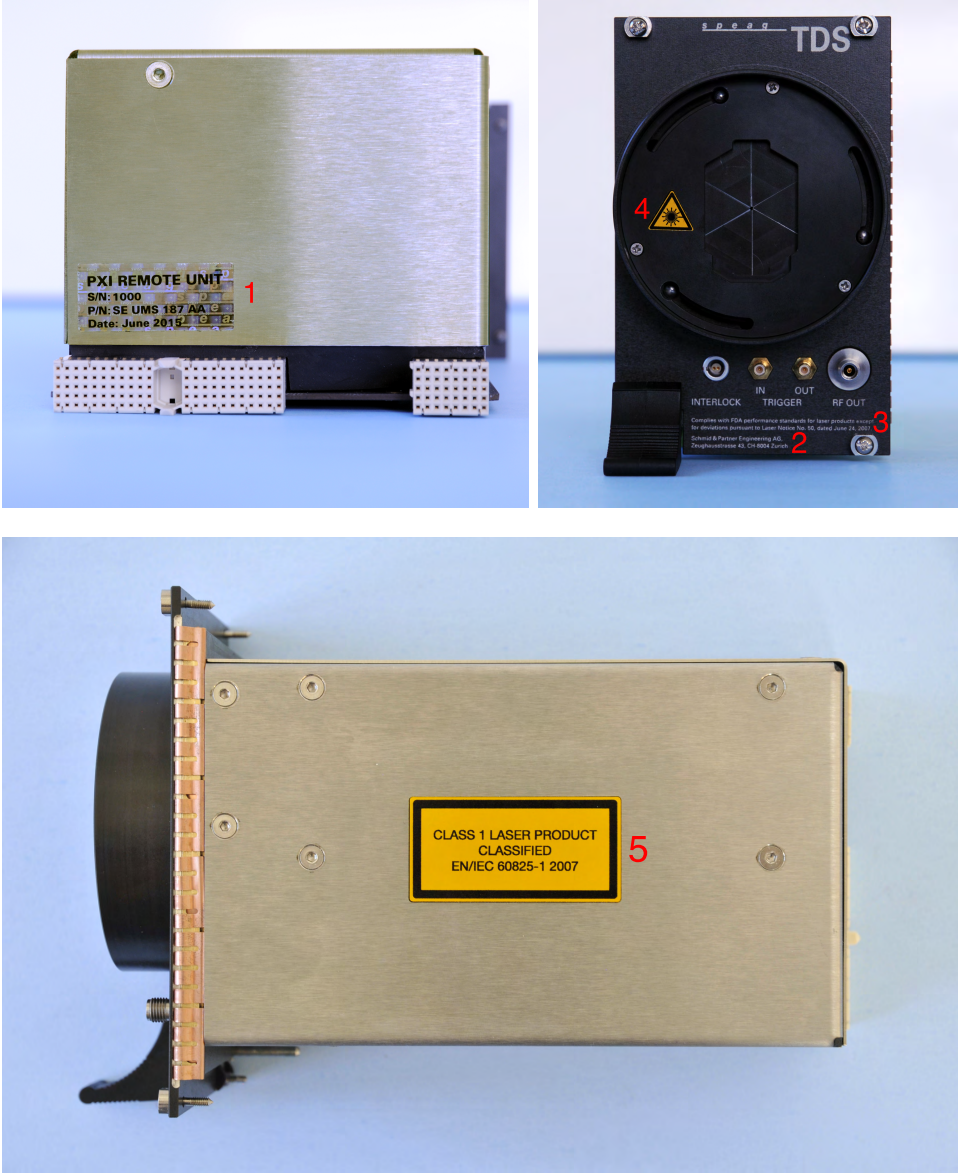
Figure 2: PXI TDS Remote Unit safety marking
