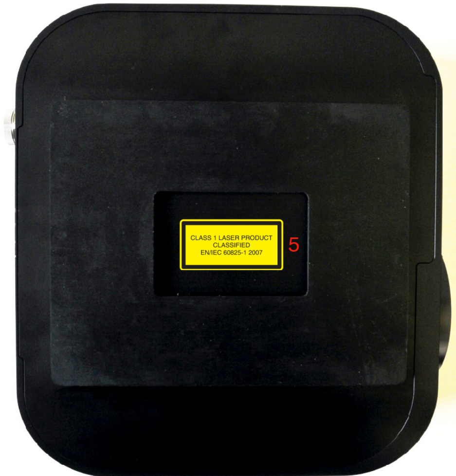
Figure 1: Standalone TDS Remote Unit safety marking
